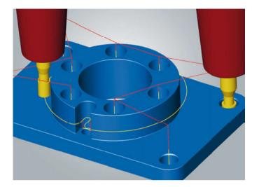
hyperMILL® JIG Grinding offers easy-to-program CAM strategies to create safe and reliable NC programs for vertical or conical chop grinding. hyperMILL® uses the machine tool's controller cycle and can be used on grinding machines but also on hybrid machines with grinding and HSC milling function.
