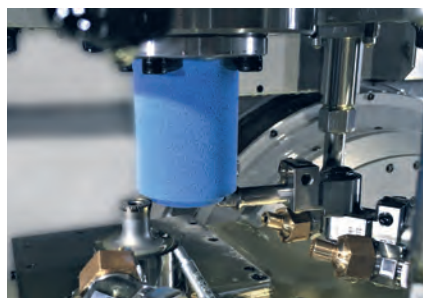
Fig. 2: Dressing the grinding wheel
