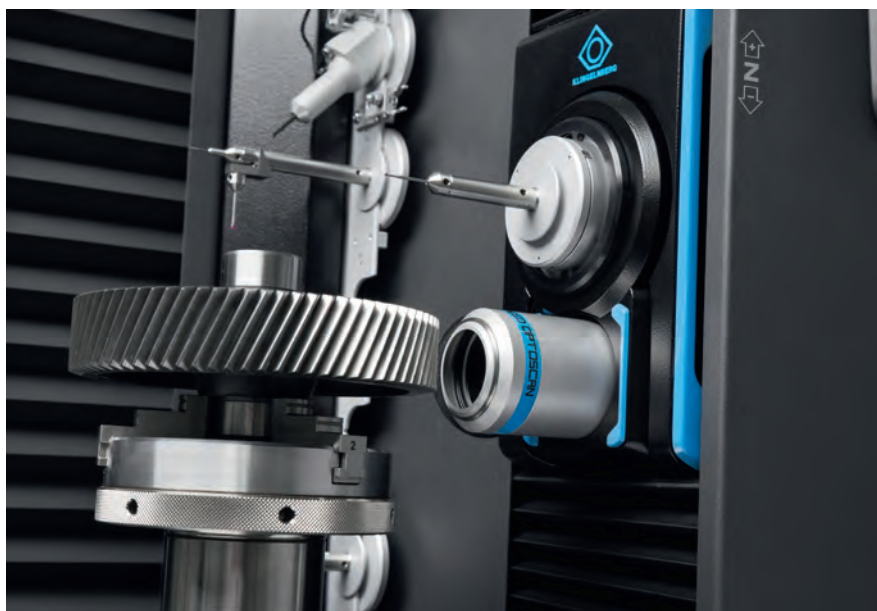
Fig. 1: Pitch Measurement with HISPEED OPTOSCAN
