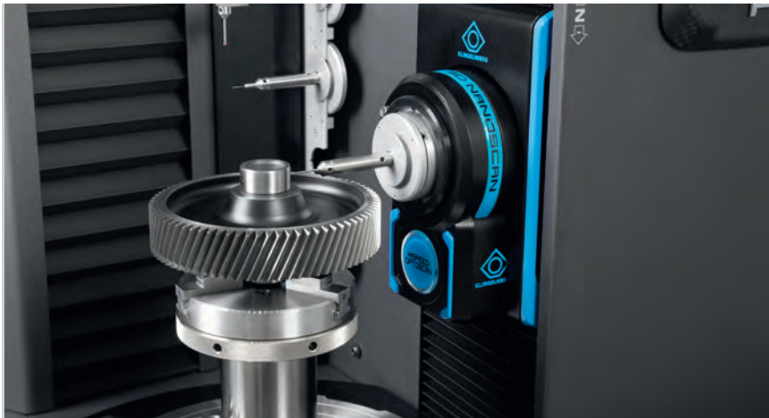
Fig. 3: Optical sensor retracted
