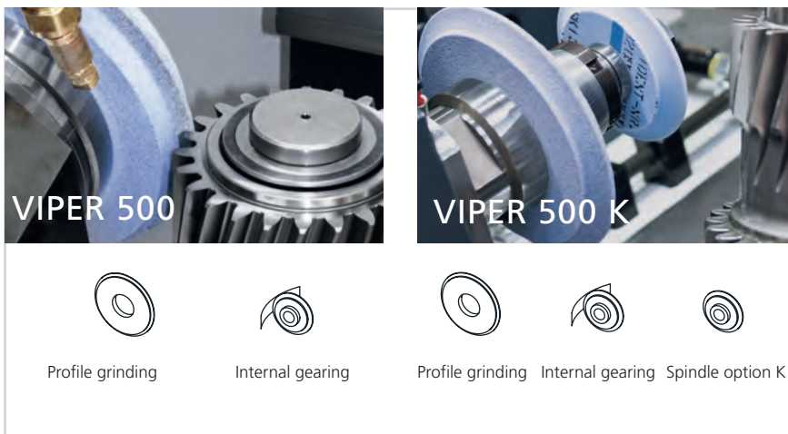
Fig. 2: Machine configuration variants 500 and 500 K
