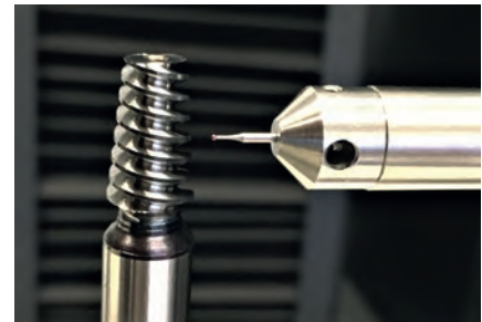
Fig. 4: Geometrical measurement of the bevel pinion
