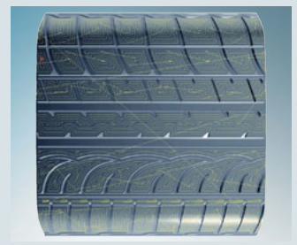
Segment toolpaths are generated using the tire clock.
