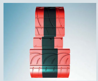
The tire module creates the required geometries for pitch and pitch-combination programming.
