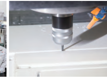
Machining parts for semiconductor manufacturing equipment using a 5-axis machine
