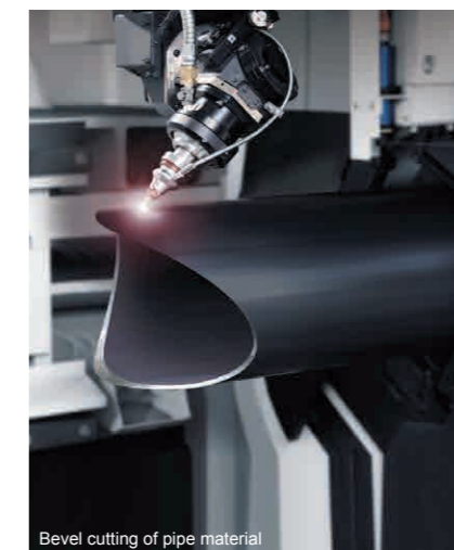
Bevel cutting of pipe material
